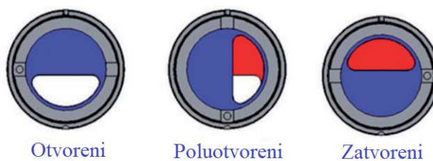
Slika 2-5. M-I Swaco SuperChoke tri položaja zapornog elementa tipa ploče s unaprijed urezanim otvorima ( https://www.slb.com/-/media/files/mi/product-sheet/superchoke )
