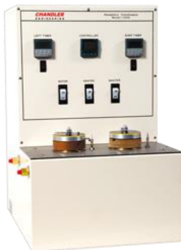
Slika 5-7. Atmosferski konzistometar (Chandler Engineering, 2019)
