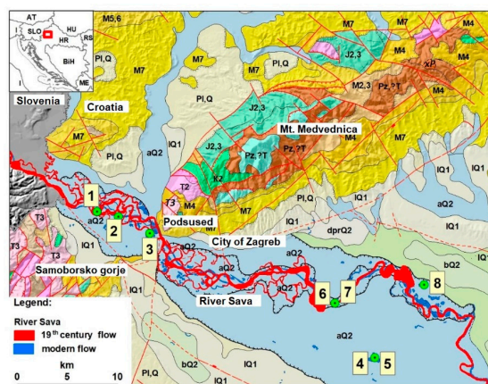
Figure 1. Geographical location and map of the study area. Sava River watercourses: non-regulated (red) and regulated (blue), sampling locations (green dots: 1–8): 1—Samobor; 2—Savršćak; 3—Orešje; 4—Novo Čiče1; 5—Novo Čiče 2; 6—Novi Petruševac 1; 7—Novi Petruševac 2; 8—Ivanja Reka. Modified from [18]. Legend for geology, from [19]: xP—Permian (magmatics: quartz diorites, granodiorites); Pz?T–P—Palaeozoic to Triassic (parametamorphites); T2—Middle Triassic (carbonates, clastic, and pyroclastic deposits); T3—Norian to Rhaetian (dolomites); J2,3—Middle to Upper Jurassic (ophiolites); K2—Upper Cretaceous (carbonate clastics and “Scaglia” limestones); M2,3—Ottomanian to Carpathian (clastics, carbonates with clastics); M4—Badenian ( Lithothamnium limestones and similar rocks); M5,6—Sarmatian to Pannonian (carbonate clastics); M7—Pontian (clastics and coal); Pl,Q—Plio-Quaternary (clastic deposits); IQ1—Pleistocene (loess sediments); dprQ2: Holocene (diluvial and proluvial sediments); aQ2—Holocene (fluvial deposits); bQ1—Holocene (pond deposits).
