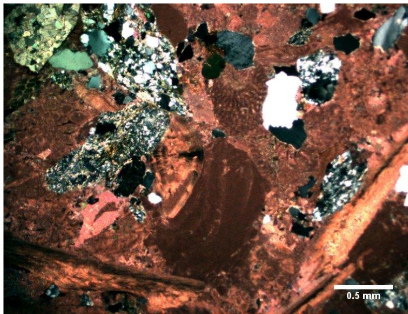
Figure 5. A photomicrograph of the typical Middle Miocene (Badenian) calcarenite from northern Croatia (Breznički Hum locality), stained with alizarin red.
