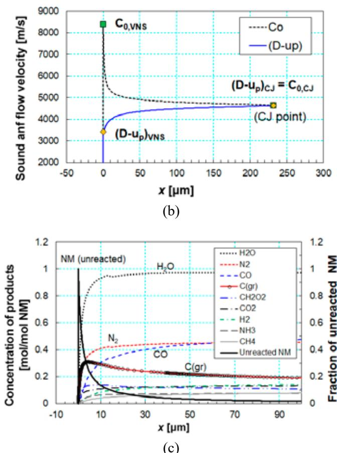
**Figure 8.** Spatial distribution of pressure and temperature (a), sound and flow velocity (b), and concentration of products within first 100  $\mu\text{m}$  (25) behind the shock (c); calculation done using PB-C1.7D2 rate model
