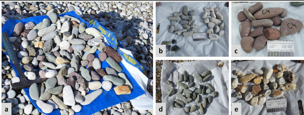
Figure 3: Bulk sample of gravels (a) and clast sorted into categories: (b) – carbonates; (c) – red sandstones; (d) – green sandstones; (e) – quartz(ites) and cherts. Collected in gravel pit "Abesinija" in March 2020.
