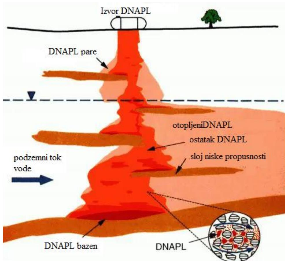
Slika 5.3. Kretanje gustih organskih spojeva kroz podzemlje ([www.vertexeng.com/dense-non-aqueous-phase-liquid-contamination](http://www.vertexeng.com/dense-non-aqueous-phase-liquid-contamination))
