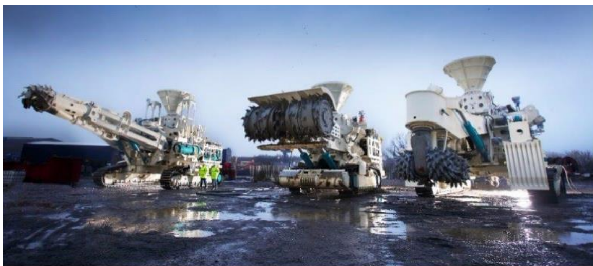
Slika 4-3. Strojevi Nautilus minerals (Cherkashov, 2017)
