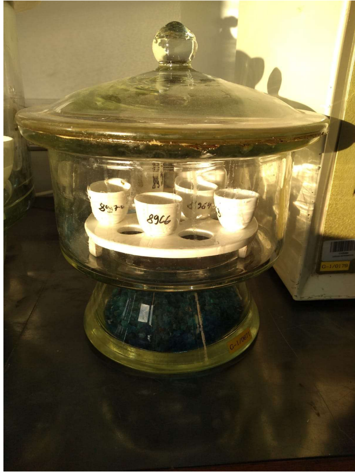
Figure 3-18. Samples cooling in a desiccator after drying
