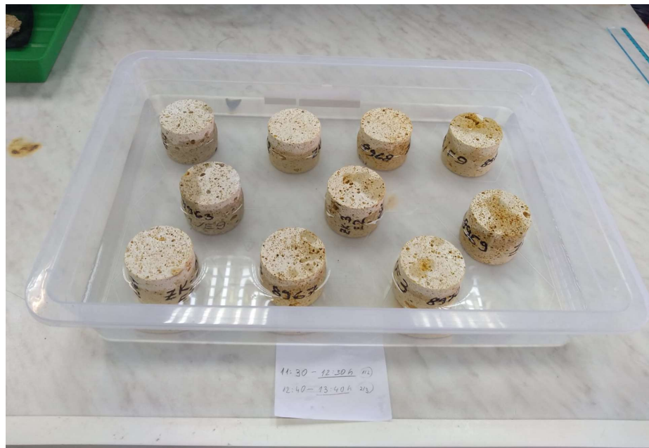
Figure 3-25. Test samples resting in water 2/3 of their height
