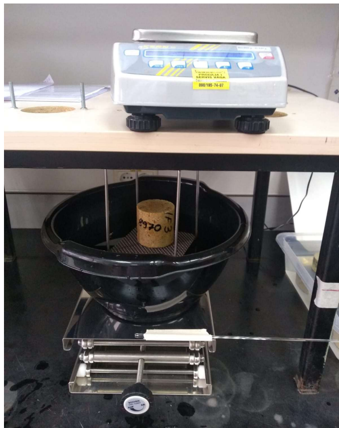
Figure 3-31. Sample 8970 being placed on setup for measuring the sample's weight under water ( m_h )
