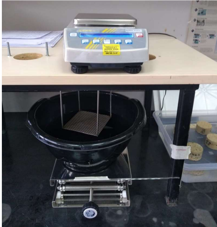
Figure 3-30. The setup for measuring the sample's weight under water ( m_h )
