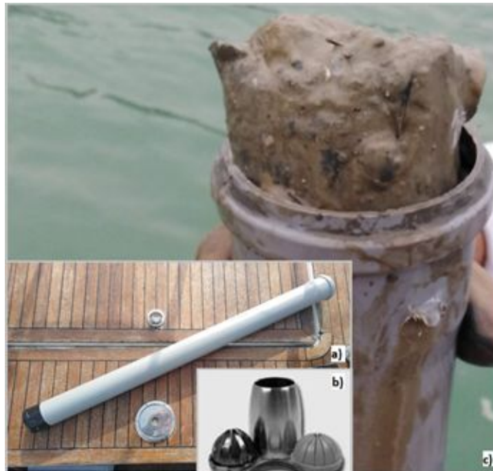
Figure 3: A hand core sampler (a) with one way valve (b) showing retrieved sediment (c).
