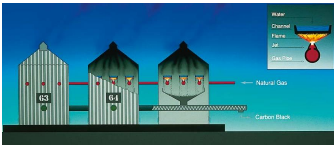
Figure 6-6. Schematic of channel black production process (Orion Engineered Carbons, 2015).
