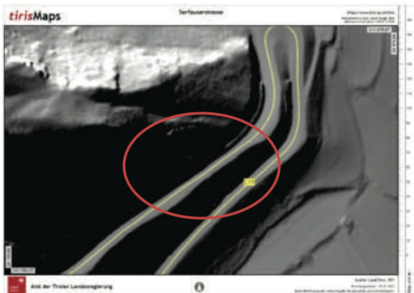
Figure 6 Detail of the digital terrain map showing unstable slope features, with the ring indicating the slope failure of the Serfauserstrasse in winter 2018 (tirisMaps 2014).
