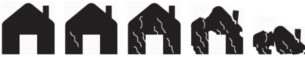
Fig. 3 Typology of most common object damage classification: negligible; negligible to slight; moderate; prone to collapse; destroyed
