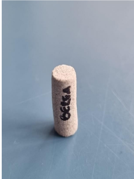
Figure 3-3. Drilled Berea sandstone sample.
