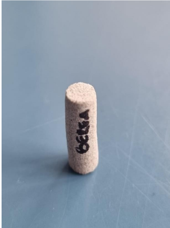
Figure 3-3. Drilled Berea sandstone sample.
