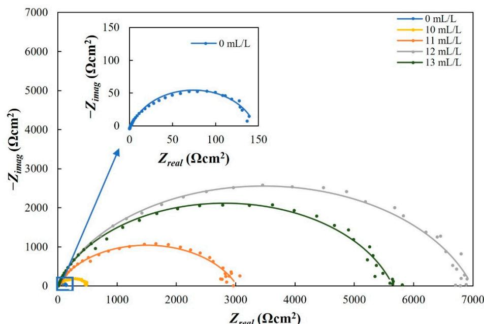
**Figure 5.** Nyquist plot scanned on the carbon-steel sample in the simulated brine saturated with  $\text{CO}_2$  with and without the inhibitor in static conditions (Adapted from [24]).
