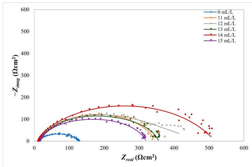
**Figure 7.** Nyquist plot scanned on the carbon-steel sample in the simulated brine saturated with CO<sub>2</sub> with and without the inhibitor in flow conditions (Adapted from [24]).
