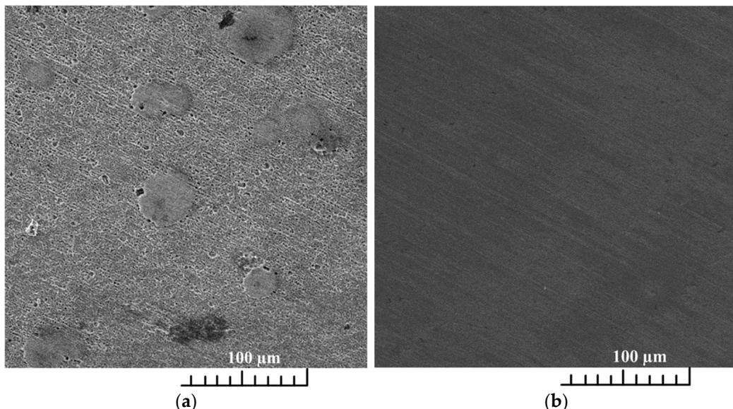
**Figure 11.** SEM scan of the carbon-steel sample after 4 h in the simulated brine saturated with CO<sub>2</sub> (a) without the extract and (b) with 12 mL/L of the extract (Adapted from [24]).
