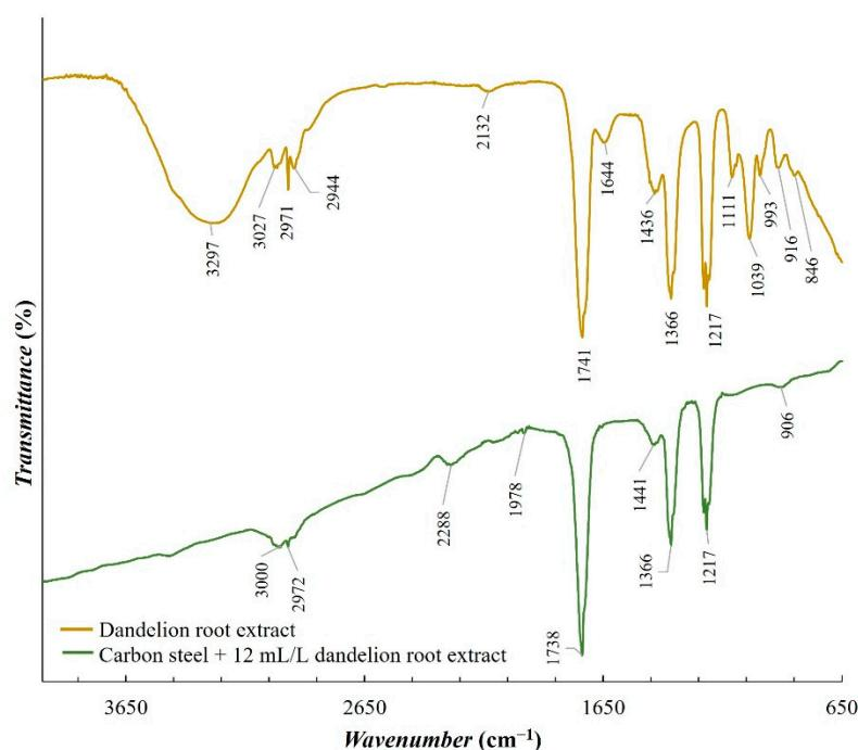
**Figure 12.** FTIR spectra of dandelion-root extract and the carbon-steel sample after 4 h of immersion in the simulated brine saturated with CO<sub>2</sub> with 12 mL/L of the extract (Adapted from [24]).
