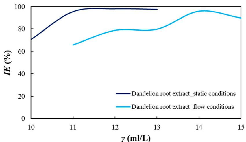
**Figure 10.** The inhibitor efficiency comparison determined from EIS scanned on the carbon-steel sample in the simulated brine saturated with CO<sub>2</sub> (Adapted from [24]).
