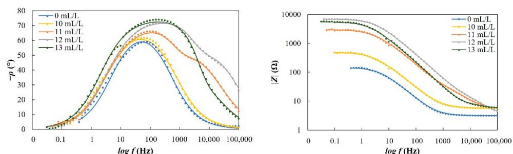
**Figure 6.** Bode plots scanned on the carbon-steel sample in the simulated brine saturated with  $\text{CO}_2$  with and without the inhibitor in static conditions (Adapted from [24]).
