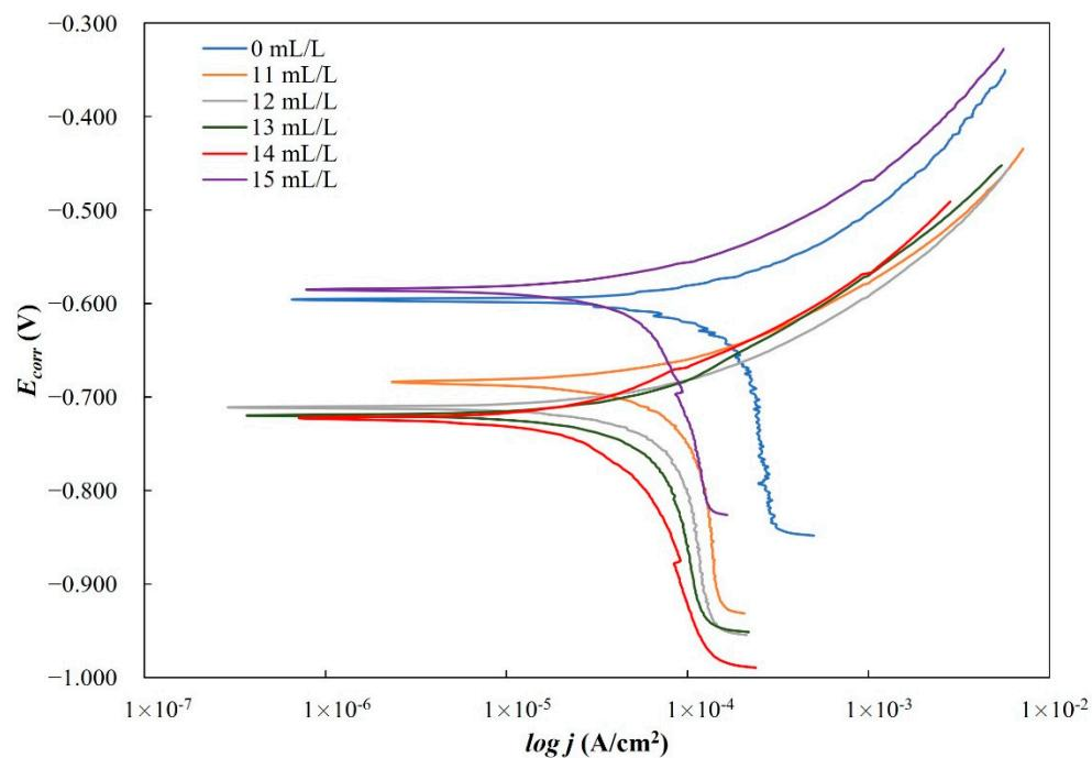
**Figure 3.** Polarization curves scanned on the carbon-steel sample in the simulated brine saturated with CO<sub>2</sub> with and without inhibitor in flow conditions (Adapted from [24]).
