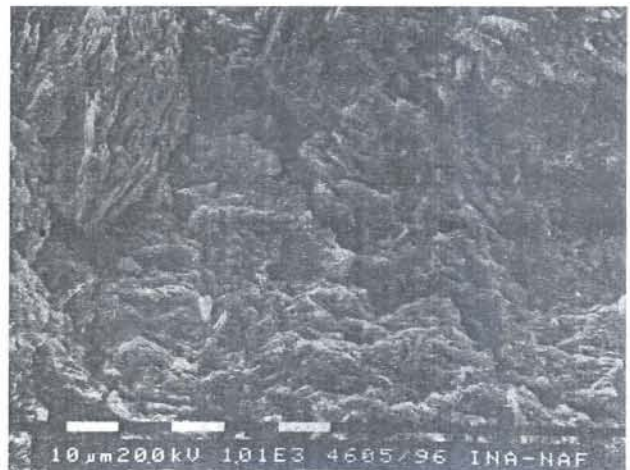
Fig. 6. Surface of spiltized diabase following the fracturing of the sample (bar = 10 μm). Microfractures of this kind are considerably less frequent in diabase compared to andesite, and which are not only of tectonic origin.
