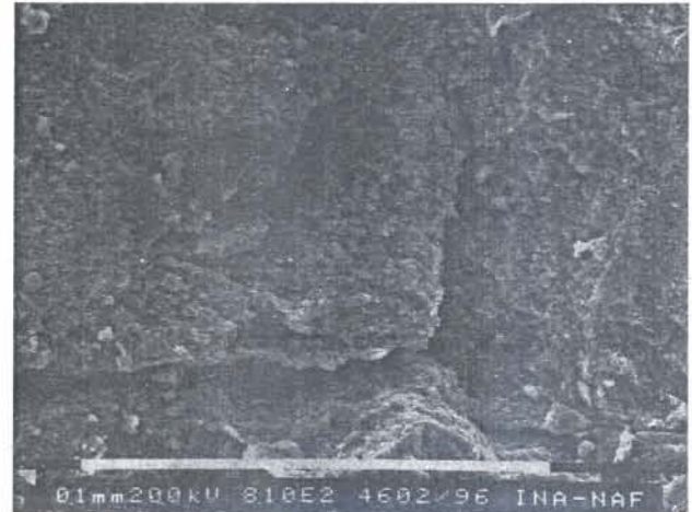
Fig. 4. Surface of the andesite sample following fracturing (bar = 10 μm) and the compression strength test. Strongly outlined microfractures and freshly formed intercrystal porosity among
