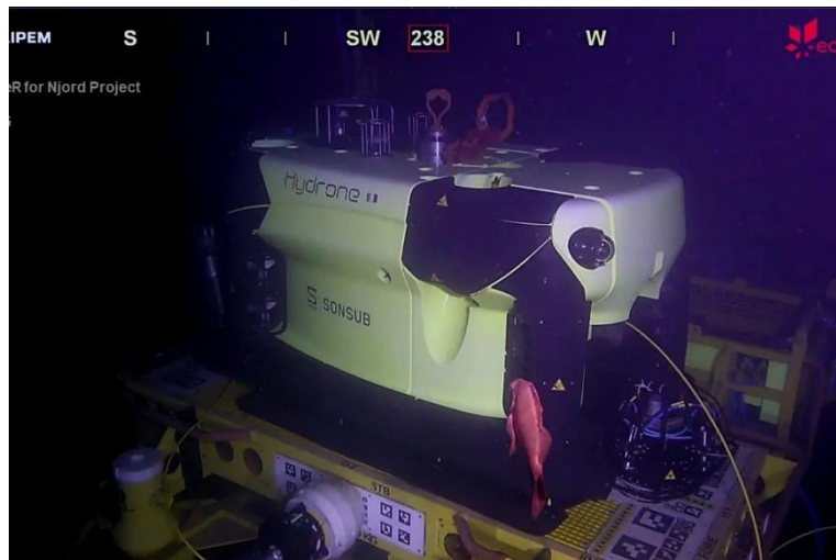
Slika 4-3. Equinorov Saipem Hydrone-R podvodni dron (Equinor, n.d.c)
