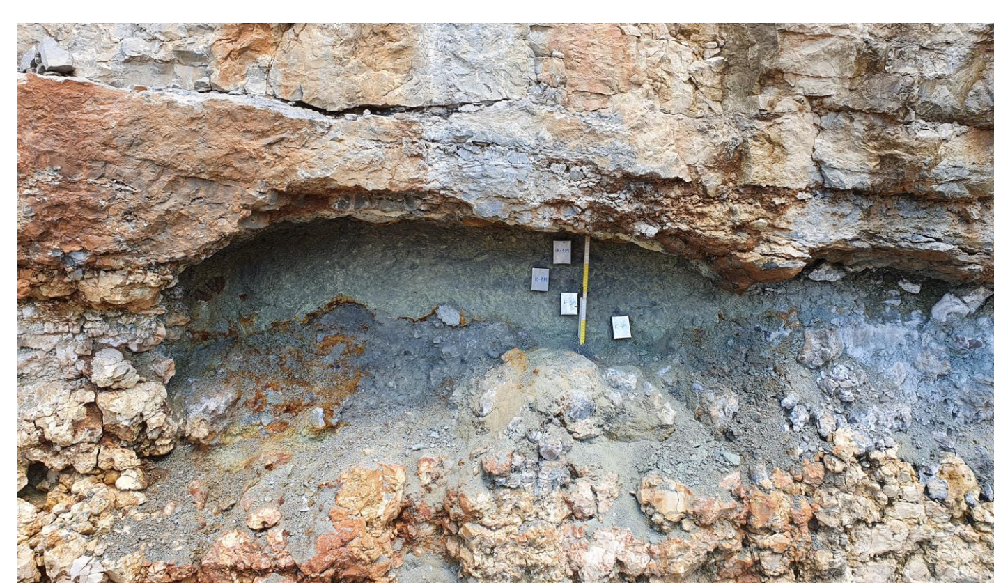
Fig. 4. Profile of greenish-grey clay in Kanfanar quarry with Kubiena boxes.
