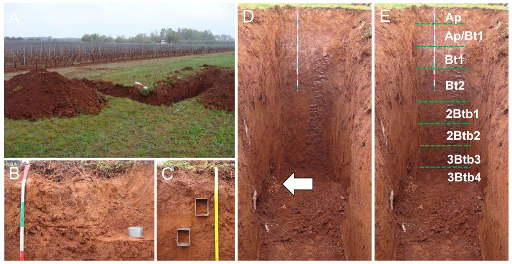
a) RPS located in a vineyard at Koreniki (west coast of the Istrian peninsula, Croatia); b) Sampling of undisturbed soil from Ap/Bt1 horizon using 100 cm<sup>3</sup> core. c) Positions of Kubiena boxes in Ap and Ap/Bt1 horizons. d) Cleaned soil profile situated on a Lower Eocene limestone (see white arrow); e) Soil profile with Ap, Ap/Bt1, Bt1, Bt2, 2Btb1, 2Btb2, 3Btb3 and 3Btb4 horizons.
