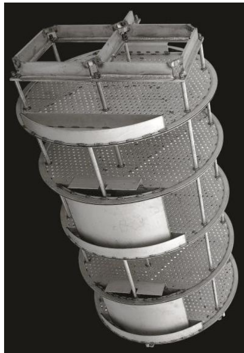
Figure 2-7 A stack of sieve trays of an absorption column (University of Michigan, 2024)
