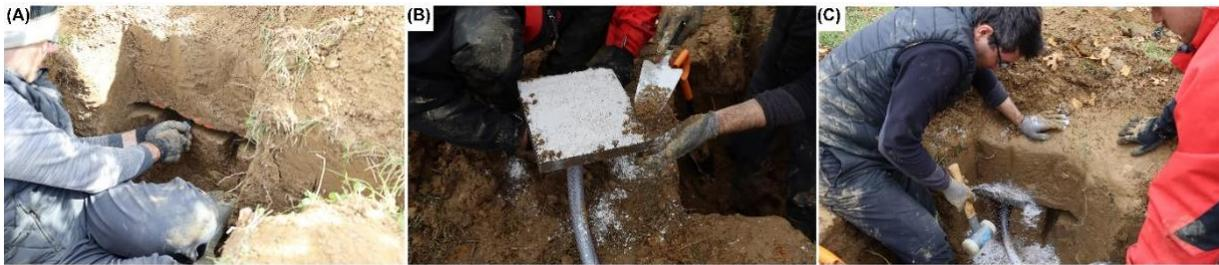
**Figure 3.** Process of installation of passive wick lysimeters: (A) precision cutting, (B) lysimeter assembly and application of crushed soil and quartz flour, and (C) positioning the lysimeter with a hammer at the SUPREHILL Critical Zone Observatory (CZO).
