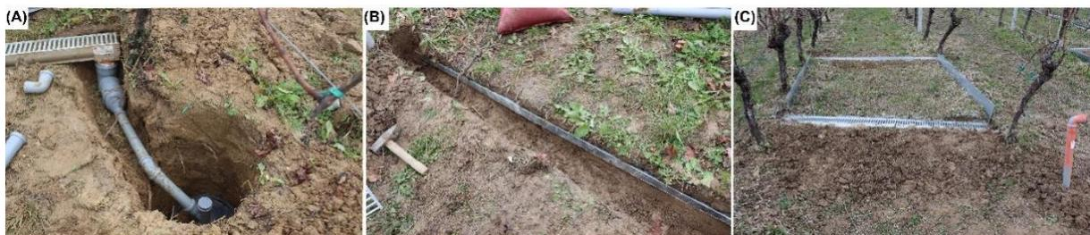
**Figure 4.** Process of installation of surface runoff collection instruments: (A) collection tank placement and pipe connection, (B) flow guide placement (C) border and drain channel placement at the SUPREHILL Critical Zone Observatory (CZO).
