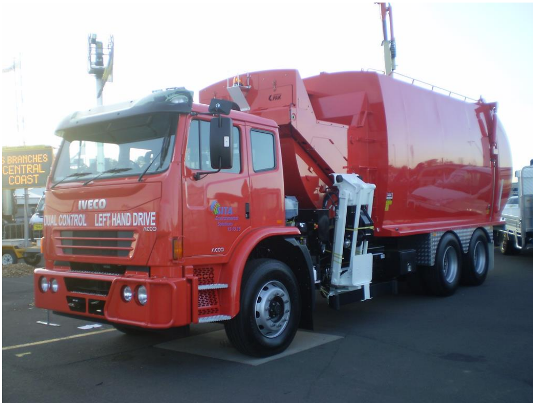
Figure 9-3. A Raptor Side Lift truck; note the side lift mechanism on the truck to lift the plastic containers (Mitch, 2011).
