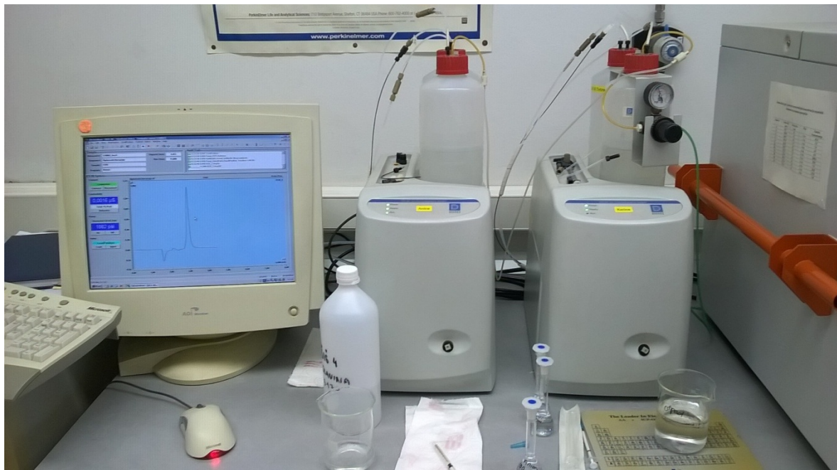
Slika 3.4 Ionski kromatograf ( ICS-1000 Ion Chromatography System, Dionex )
