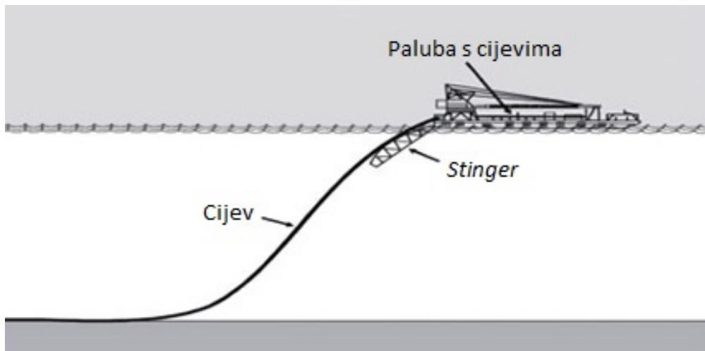
Slika 2-11. S-polaganje cjevovoda ([www.rigzone.com](http://www.rigzone.com))
