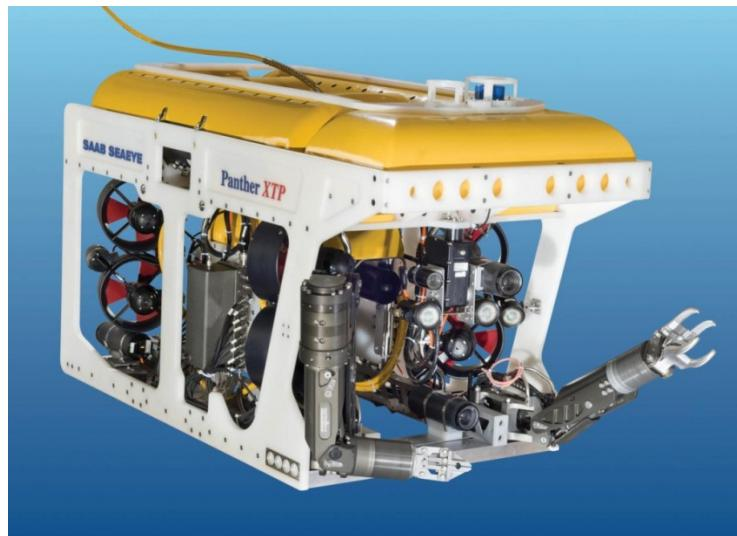
Slika 2-3. Daljinski upravljana jedinica (*engl. Remotely Operated Vehicle – ROV*)
