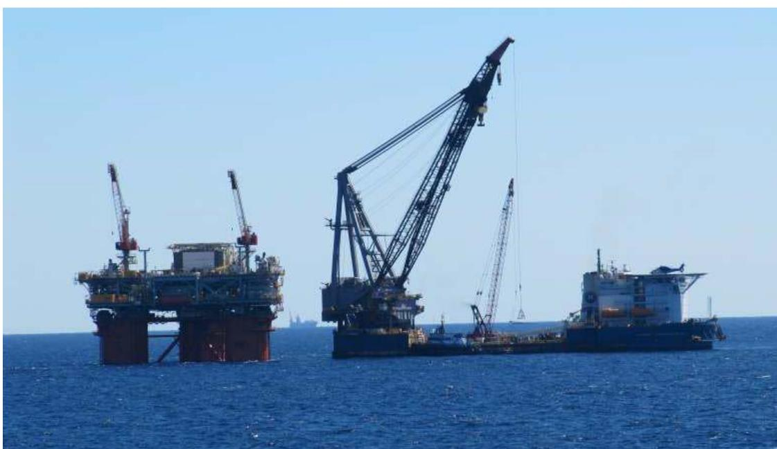
Slika 2-8. Barža s rotirajućom dizalicom (desno) ([www.shipspotting.com](http://www.shipspotting.com))
