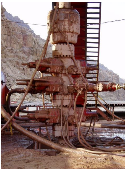
Slika 7-1. Preventerski sklop ( http://www.iwcfdrillengineer.com )
