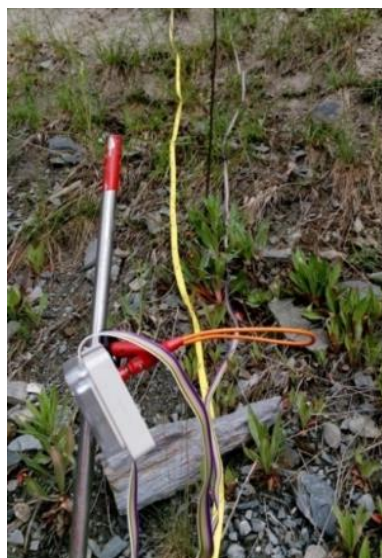
Figure 5-4 Field photo showing example of installed electrode
