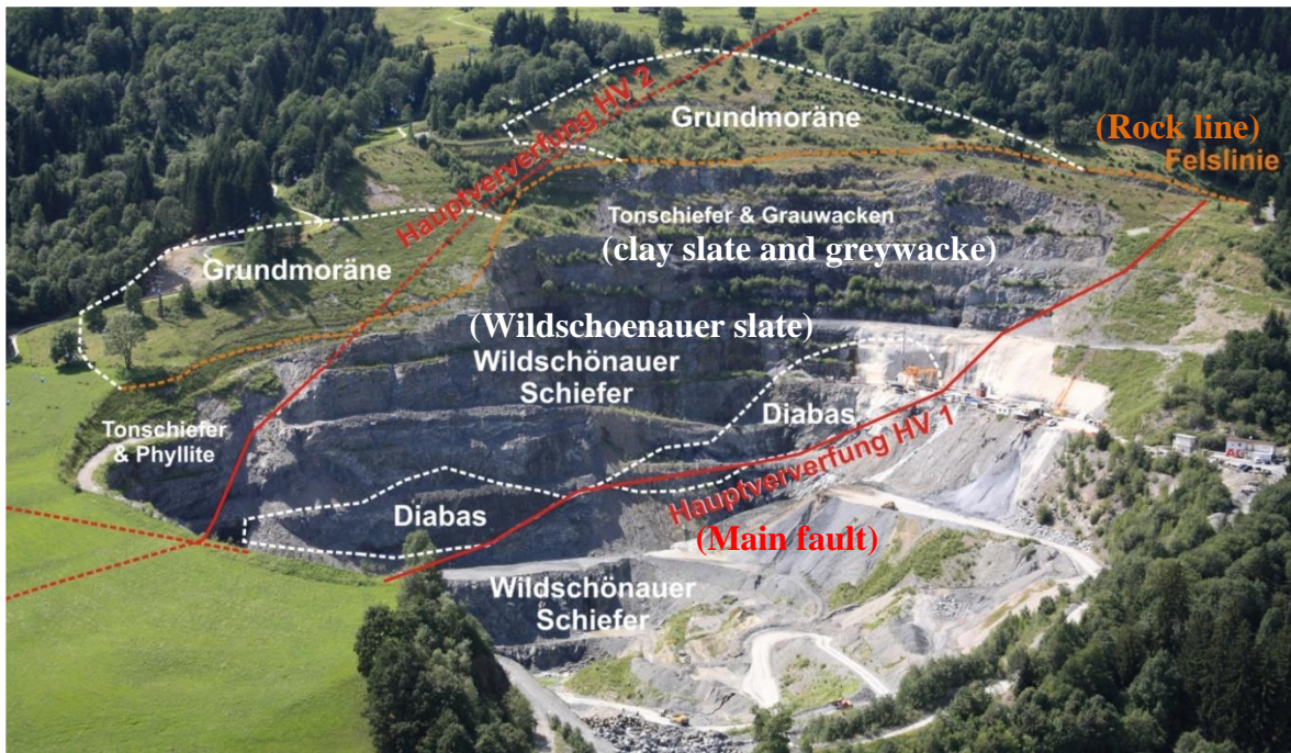
Figure 4-2 View of the Hinterburg opencast mine from the east with the most important geological formations and two main disturbance zones (Anthes et al., 2011)
