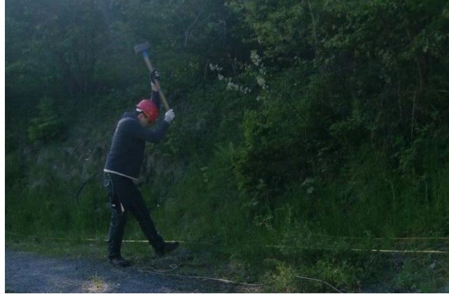
Figure 5-7 Hammer shooting at the beginning of the profile P1 (22 nd May, 2017)
