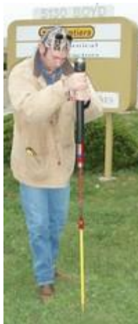
Slika 5.1: Sonda Model 204 (GeoFrontiers, 2018)
