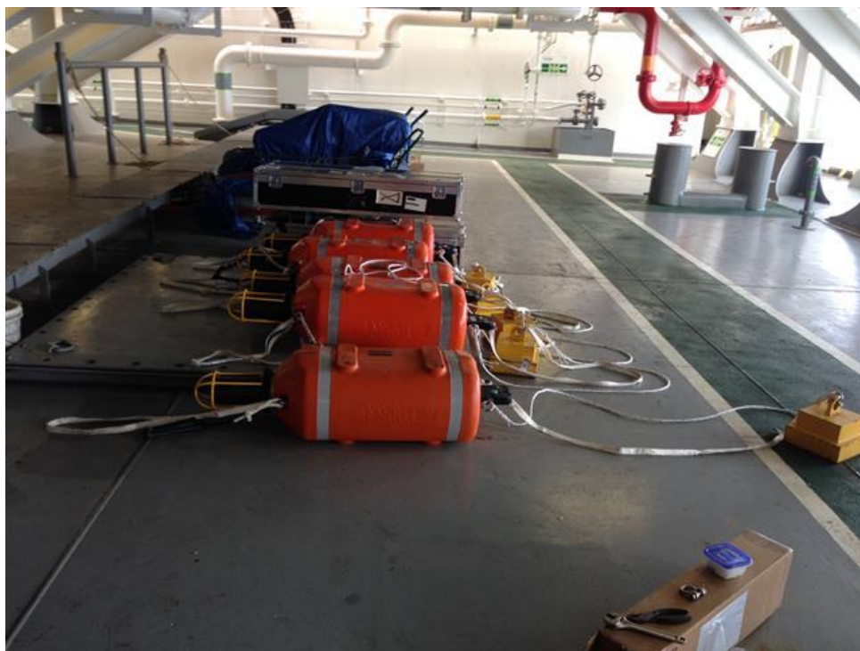
Slika 3-7. Transponderi (Pacific Drilling, 2009)
