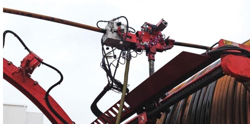
**Slika 4-10.** Mjerač duljiine tubinga (Drilling Contractor, 2018)
