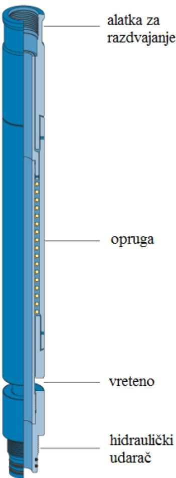
**Slika 5-17.** Mehanički udarač (škare) (Schlumberger Oilfield Glossary, 2018c)
