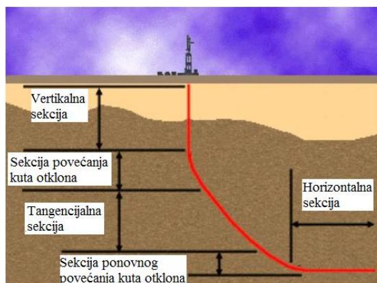
Slika 1-1. Dijelovi kanala horizontalne bušotine (Directionaldrilling.wordpress.com, 2015)
