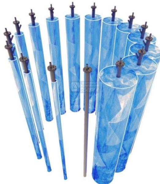
**Slika 2-23** Shema zaledivanja tla oko cijevi (Artificial ground freezing technique is used to construct substructures in soft, unstable water-bearing soils, 2019)
