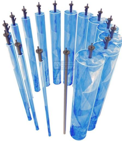
Slika 2-23 Shema zaleđivanja tla oko cijevi (Artificial ground freezing technique is used to construct substructures in soft, unstable water-bearing soils, 2019)
