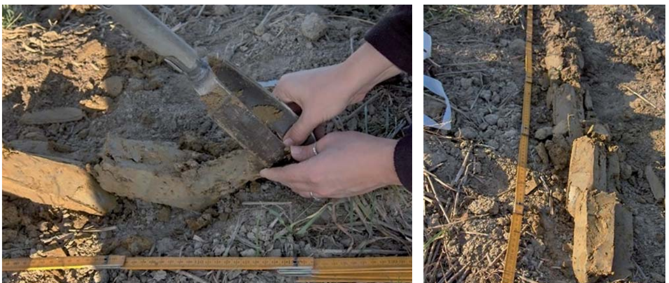
Figure 3. and 4. Soil sampling by probe
