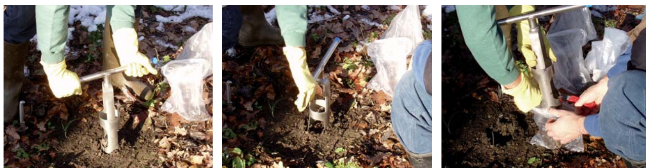
Figure 5. Sampling of mineral layer of soil
