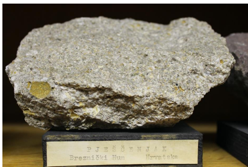
Figure 4. A sample of typical Middle Miocene (Badenian) calcarenite from northern Croatia (Breznički Hum locality). Collection of the Faculty of Mining, Geology and Petroleum Engineering.
