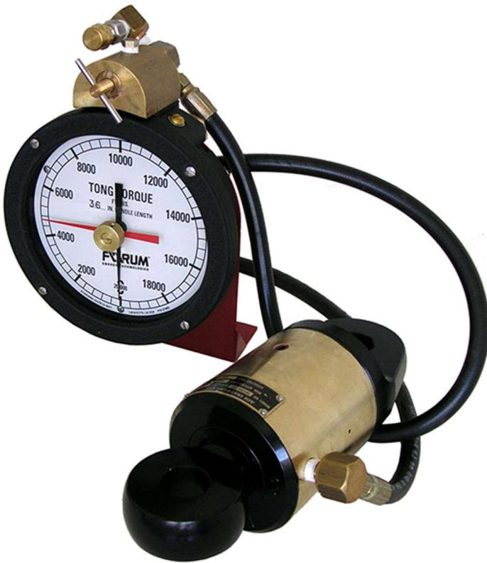
**Slika 2-11.** Dinamometar (Forum Energy Technologies, 2020 c)
