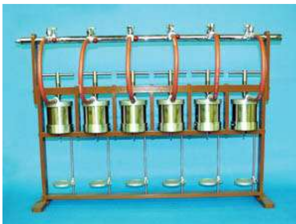
Slika 3-10. API filter preša ( http://www.ofite.com )
