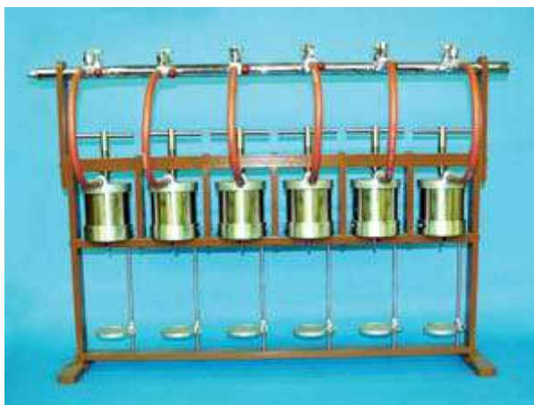
Slika 3-10. API filter preša ( http://www.ofite.com )
