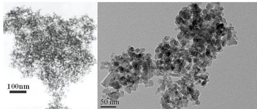
**Slika 4-2.** TEM snimke suhih nanočestica SiO<sub>2</sub> (lijevo) i nanočestica SiO<sub>2</sub> suspendiranih u vodi (desno) ([www.us-nano.com/inc/sdetail/408](http://www.us-nano.com/inc/sdetail/408) i [www.us-nano.com/inc/sdetail/626](http://www.us-nano.com/inc/sdetail/626))
