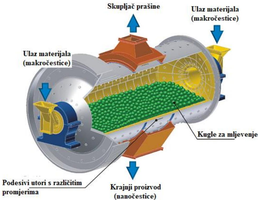
**Slika 1-3.** Kuglični mlin ([www.sherlocks.com.au](http://www.sherlocks.com.au))
