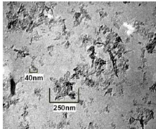
**Slika 1-6.** TEM snimka  $\text{Al}_2\text{O}_3$  nanofluida (Williams et al., 2006)
