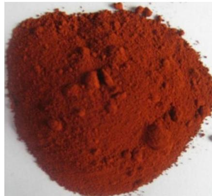
**Slika 4-5.** Nanočestice Fe<sub>2</sub>O<sub>3</sub> u obliku praha ([www.what-is-nanotechnology.com](http://www.what-is-nanotechnology.com))
