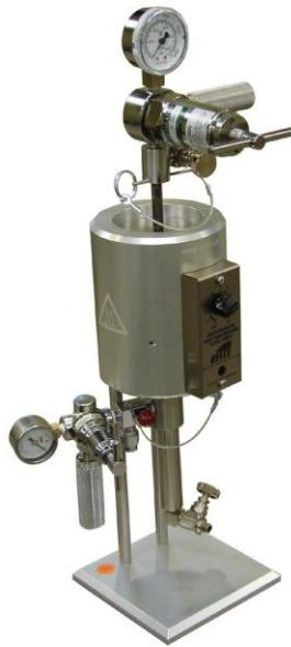
**Slika 5-8.** HTHP filter preša (OFI Testing Equipment, Inc., 2014)
