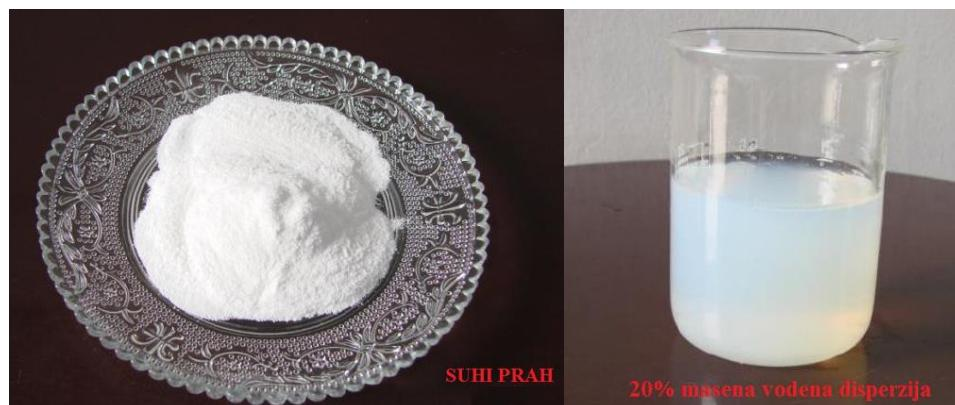
**Slika 4-3.** Nanočestice Al<sub>2</sub>O<sub>3</sub> u obliku praha (lijevo) i nanočestice Al<sub>2</sub>O<sub>3</sub> suspendirane u vodi (desno) ([www.s.b5z.net/i/u/10091461/i/US3004-big.jpg](http://www.s.b5z.net/i/u/10091461/i/US3004-big.jpg))
