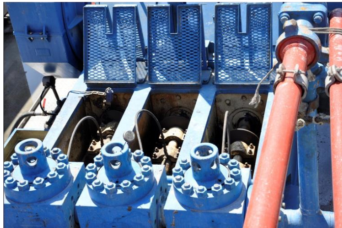
Figure 4-6. 3 cylinder mud pump ( Aydin, 2015)
