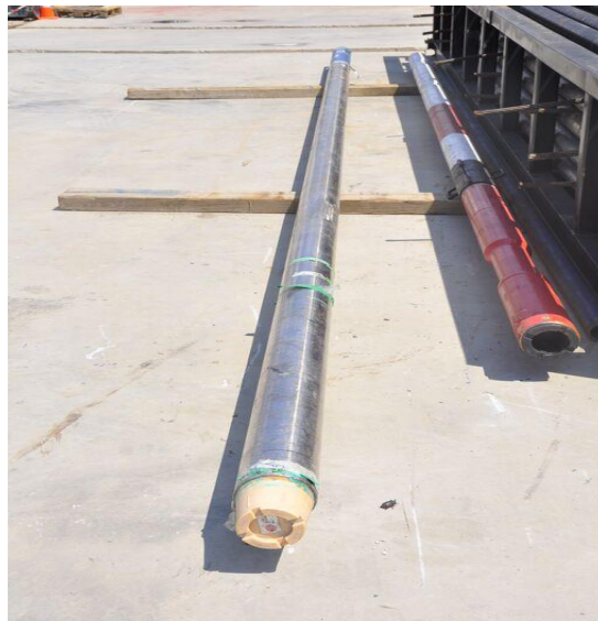
Figure 5-3. Non – magnetic drill collar (Aydin, 2015)
