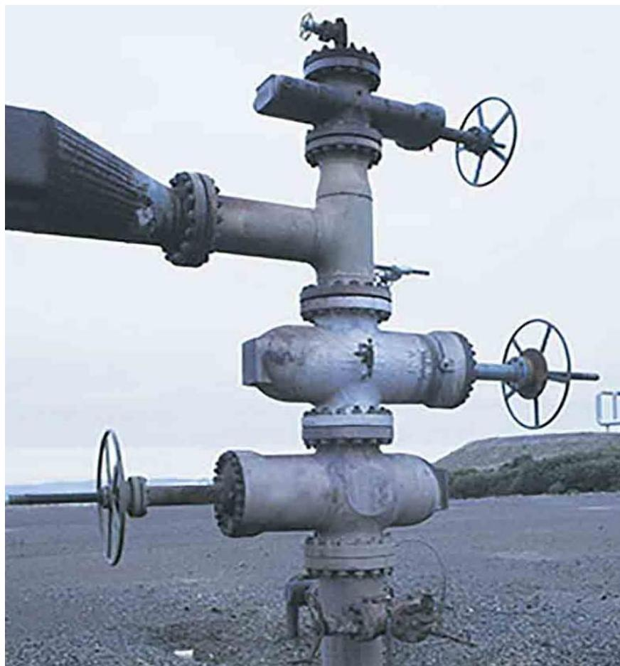
Slika 3-5. Bušotinska glava geotermalne bušotine ([www.slb.com](http://www.slb.com), 2020)
