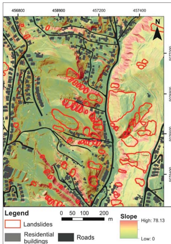
Figure 5: Landslide inventory map based on LiDAR data acquired in 2013 (Bernat Gazibara et al., 2017b). Landslides are presented on a hillshade map overlain by a transparent slope map.
