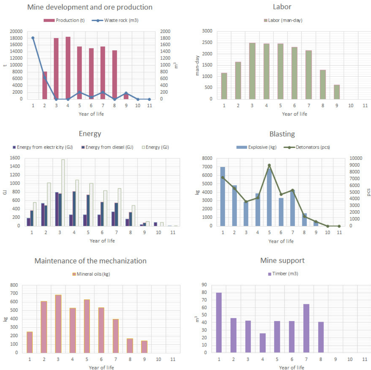
Figure 4. Life cycle inventory of mining one deposit: Mining the bauxite from the L-34 deposit in the Bauxite Mines Jajce (2010-2018). Graphs show: Mine development (m/y) and ore production (t/y); Labour (man-day/y); Energy (GJ/y); Blasting (explosive in kg/y and detonators in pcs/y); Maintenance of the mechanization (consumption of mineral oils in kg/y); Mine support (consumption of timber in m 3 /y)
