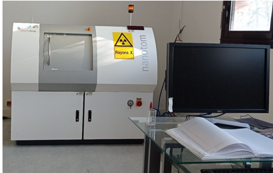
Figure 2-2. Phoenix nanotom CT device located in ISTO, France operated with General Electric (GE) acquisition and reconstruction software.
