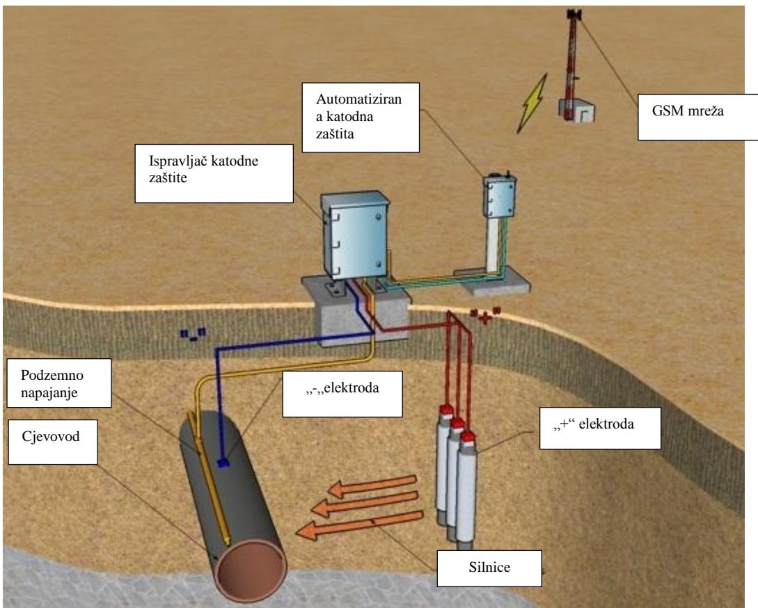
**Slika 3-4.** Katodna zaštita cjevovoda (<https://ff-automation.com/>, 2021)
