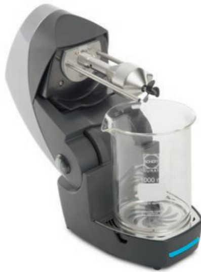
Slika 2.6 Disperzna jedinica Hydro EV (Malvern Mastersizer 3000 Brochure)
