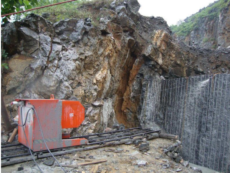
Slika 3-3: Dijamantna žična pila pri radu ( https://www.xmsinostar.com/wp-content/uploads/p2-diamond-wire-saw-machine-for-marble-quarry-cutting.jpg )
