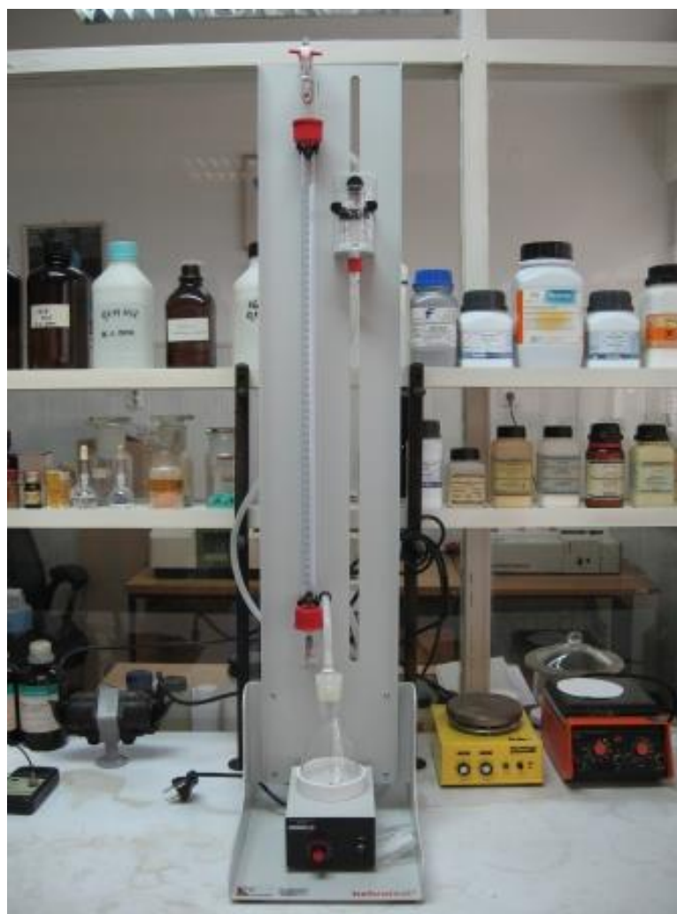
Slika 3.4. Scheibler-ov kacimeter (preuzeto s: https://sestar.irb.hr/instrumenti_show.php?ID=1263 )
