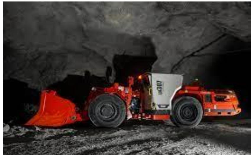
Slika 2-1. Dizelski LHD utovarivač (*Sandvik mining and rock technology*)
