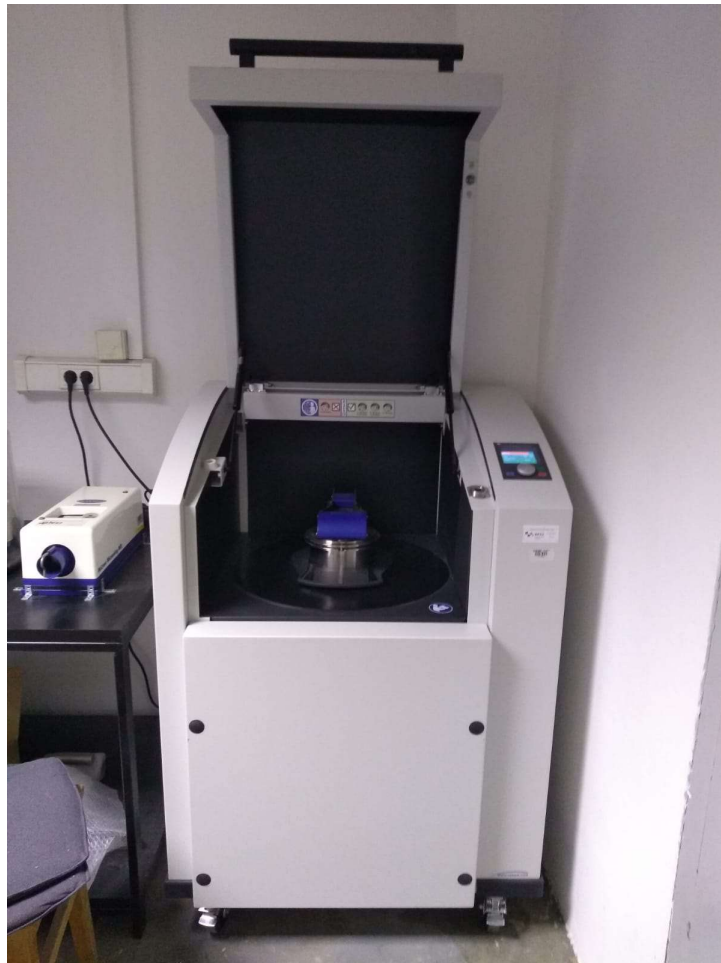
Figure 3-7. The laboratory mill used to powder the samples
