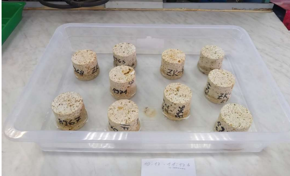
Figure 3-24. Test samples resting in water half of their height
