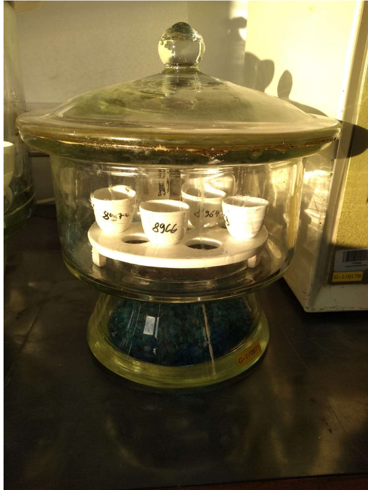
Figure 3-18. Samples cooling in a desiccator after drying
