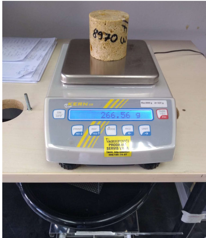
Figure 3-32. Sample 8970 weighted after being wiped with a damp cloth
