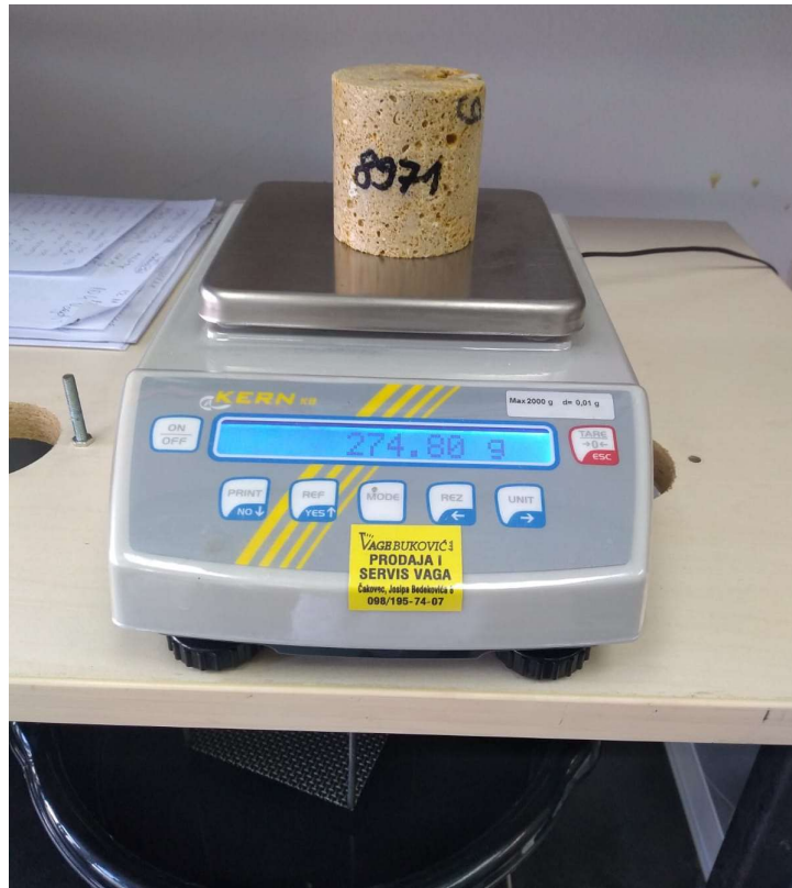
Figure 3-27. A fully saturated sample being weighted
