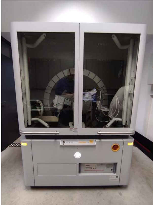
Figure 3-4. X-ray powder diffractor used in the study
