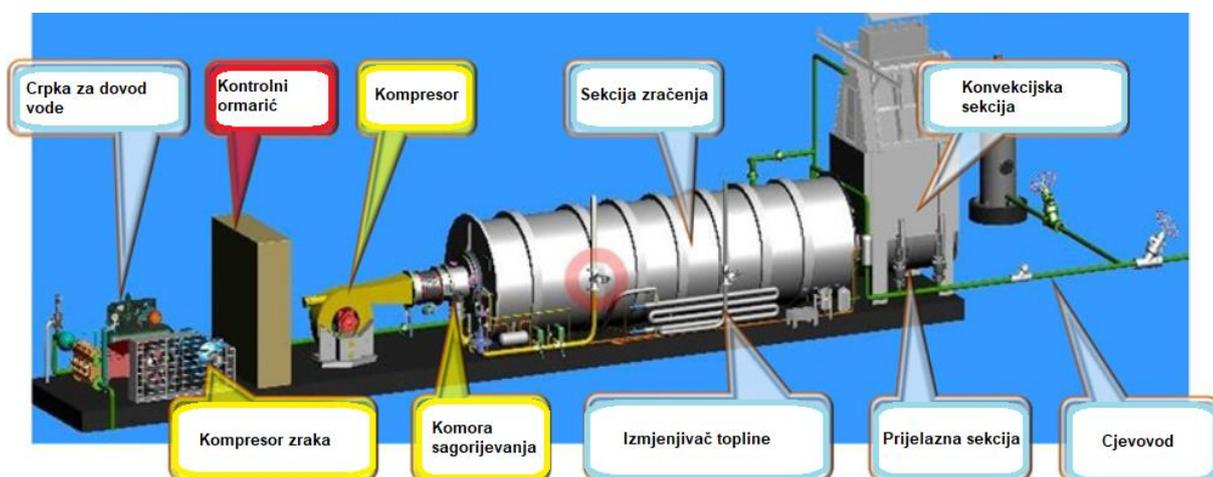
**Slika 3-8.** Dijelovi generatora mokre vodene pare ([www.enhanced-oil-recovery.com](http://www.enhanced-oil-recovery.com), 2022)
