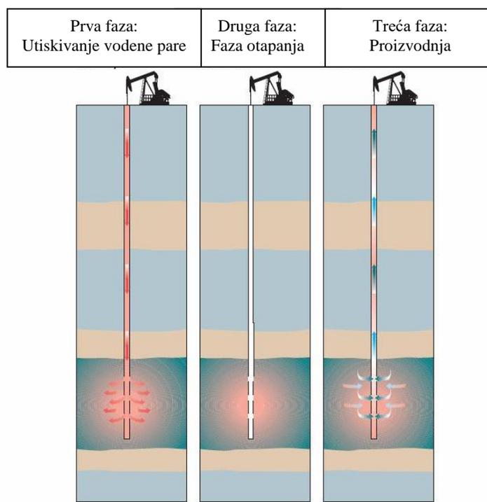
**Slika 2-1.** Faze kružnog stimuliranja vodenom parom ([www.researchgate.com](http://www.researchgate.com), 2013)
