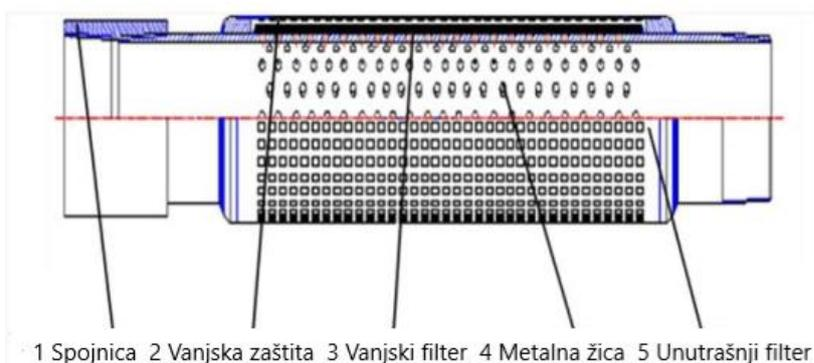
**Slika 3-10.** Filter omotan žicom (Du et al., 2018)
