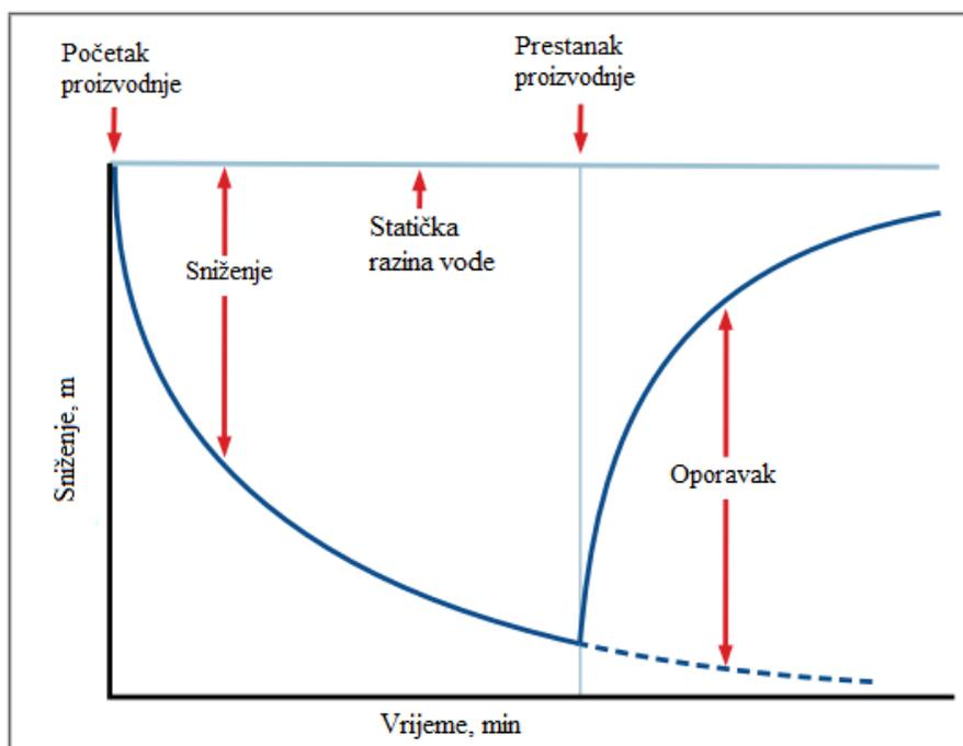
**Slika 4-5.** Prikaz mjerenja sniženja pri konstantnoj proizvodnji i povrata razine ([https://wwwguide\\_to\\_conducting\\_pumping\\_tests](https://wwwguide_to_conducting_pumping_tests), 2021)
