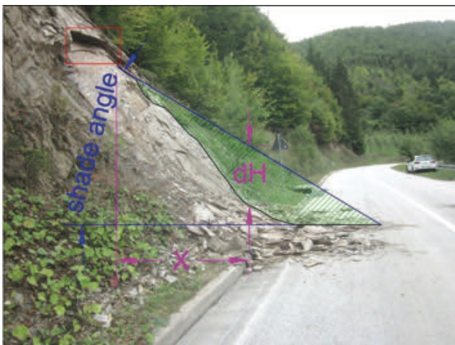
Figure 3 Cone model (red rectangle is source, black line is topographic surface, blue line is cone surface, shade angle \sim 32^\circ , green area is a trajectory domain) of 2020 event in the background (photo M. Marjanović).
