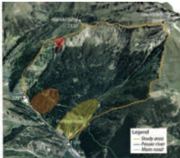
Figure 1 The Ganderberg DGSD; in red the potential rock avalanche; in orange and yellow the secondary slides.
