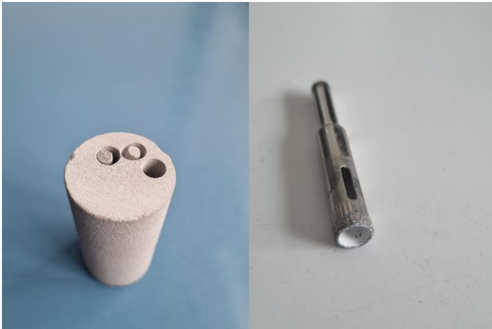
Figure 3-2. Drilled core sample (Left). The drill bit (Right).
